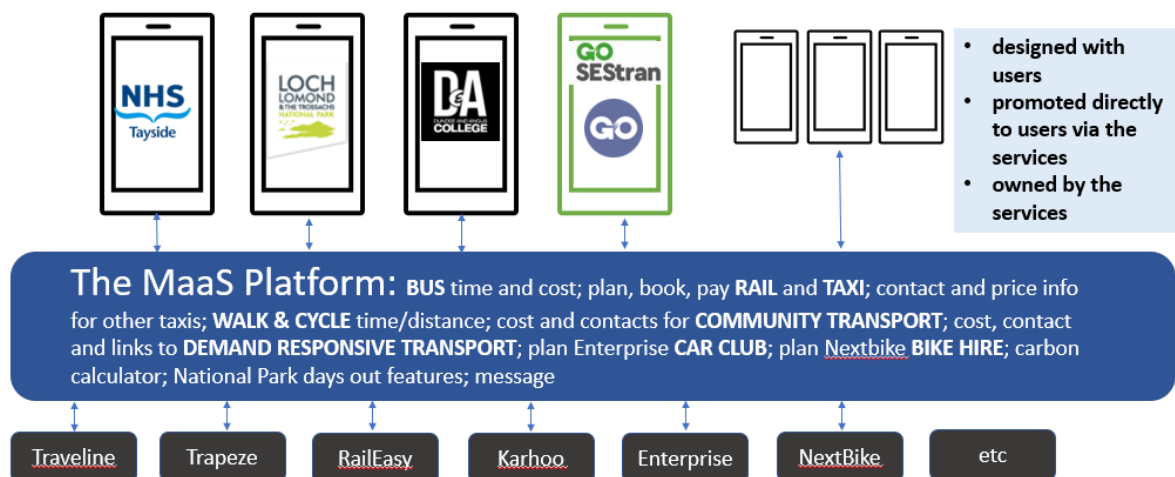
Fig 2.1: The MaaS platform, its interfaces and integrations
